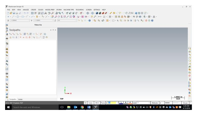
First thing is to figure out what you are making....Using the measurements from your plans, you will draw your geometry (geometry is a generic term for lines, arcs, etc. in a computer drawing program). This geometry must be drawn in the 1<sup>st</sup> quadrant of the coordinate system, so positive x and y. The placement of the geometry matters since we will later be cutting out the part using the CNC Router. The CNC Router uses the coordinates from where you draw the geometry.
